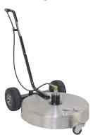
Maximum Pressure: 4000 PSI •Minimum Pressure: 1500 PSI Maximum Flow: 8 GPM •Minimum Flow: 3 GPM •Maximum Temp. 210°F. •Maximum Speed: 2000 RPM •Cleaning Path: 24" Approx. Ship Wt: 53 lbs.
